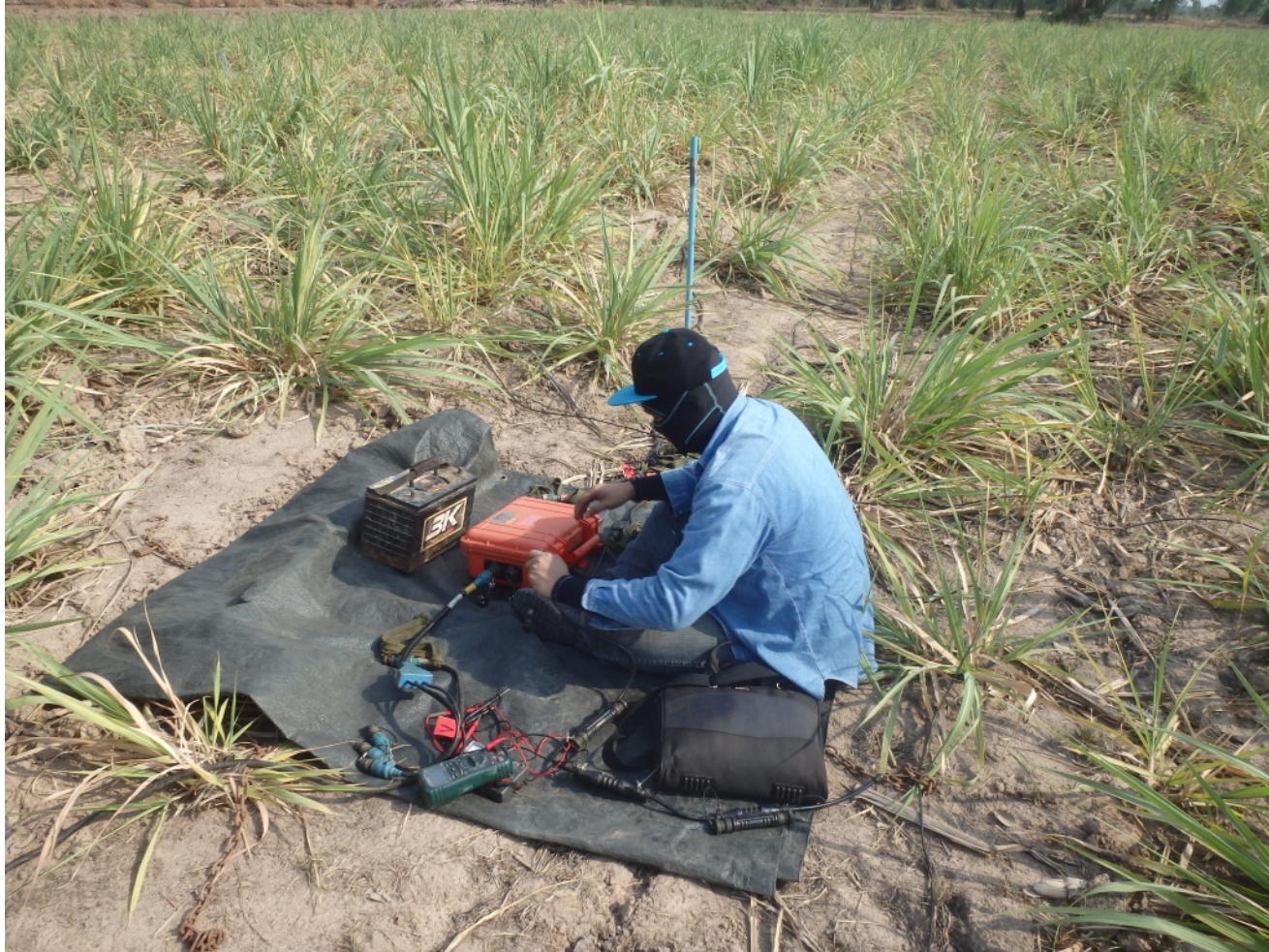
Fig. Magnetotelluric survey, somewhere in Thailand.
